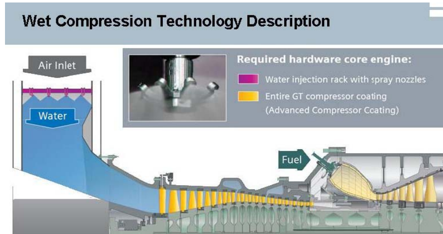
Figure 2-7: Wet Compression depiction with 100% coating of the compressor components (Al-Sati, 2014)
